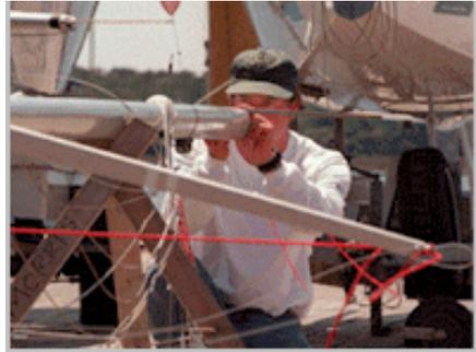
Your spreaders have a jib trim mark in the middle. If you want it seen from behind use a felt tip pen or tape and extend it to the top of the spreader as well. In winds under 18 knots the jib leech will line up with this mark. In more wind it will be slightly outside.
