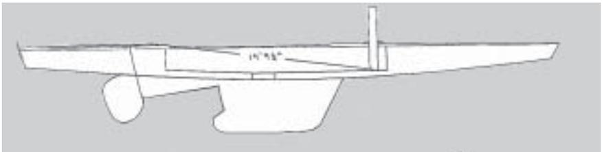
After stepping the mast, the mast butt location can be quickly checked. With the jibstay connected and backstays set, the forward edge of the outhaul boom band will be even with the stern, or slightly behind the stern. On my Folli the band is 35 mm (1.5") behind the stern. On the Mader you will find the band about even with the stern. Make sure that the mast is straight with the spreaders back and not
